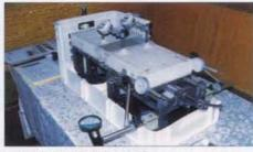
FIGURE 4 - TEST RIG TO SIMULATE CRACKING
